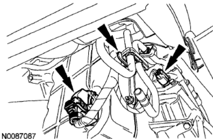
Fig. 125: Locating Transmission Electrical Connectors And Stud Bolt Courtesy of MAZDA MOTORS CORP.
