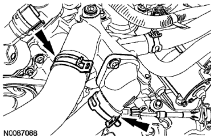
Fig. 413: Locating Upper And Lower Radiator Hoses Courtesy of MAZDA MOTORS CORP.
