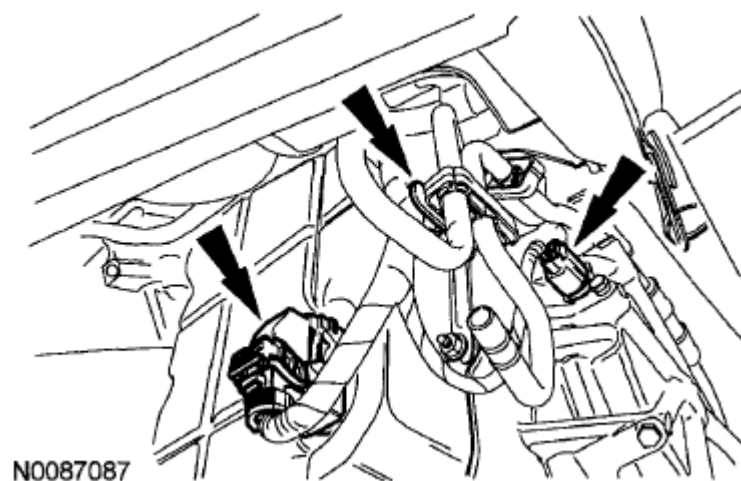
Fig. 414: Locating Transmission Electrical Connectors And Stud Bolt Courtesy of MAZDA MOTORS CORP.
