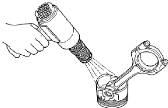
Fig. 38: Heating Piston And Connecting Rod Assembly
