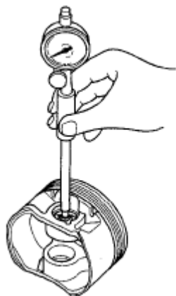
Fig. 41: Checking Difference Between Piston Pin Diameter And Piston Pin Hole Diameter Courtesy of AMERICAN HONDA MOTOR CO., INC.
