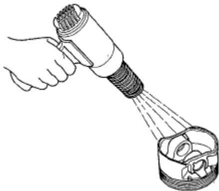
Fig. 44: Heating Piston Courtesy of AMERICAN HONDA MOTOR CO., INC.
