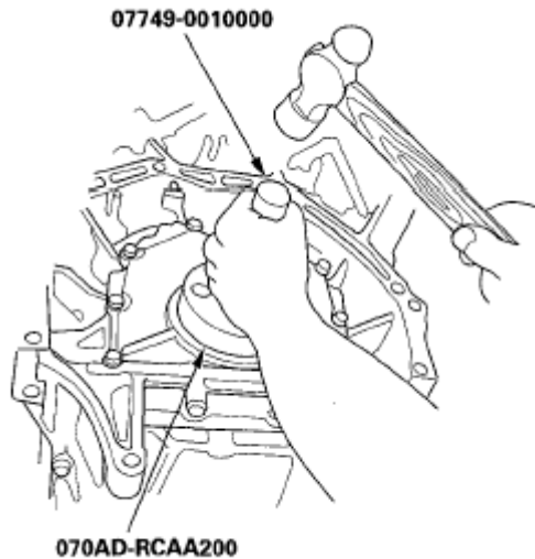
Fig. 72: Installing Transmission End Crankshaft Oil Seal Courtesy of AMERICAN HONDA MOTOR CO., INC.
