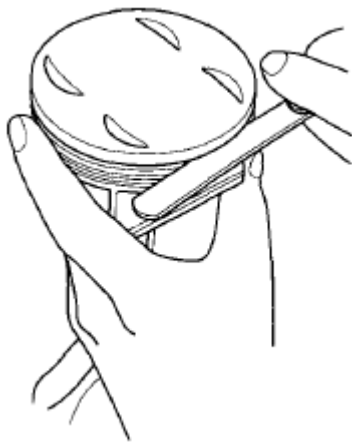
Fig. 51: Measuring Ring-To-Groove Clearance
