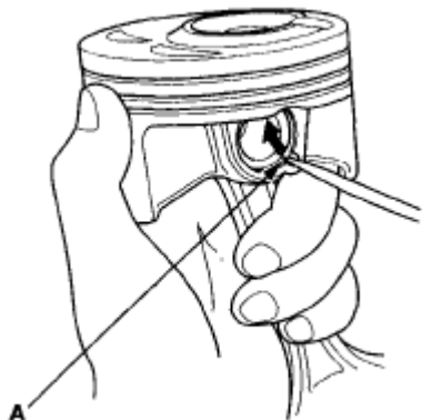
Fig. 35: Removing Snap Rings Courtesy of AMERICAN HONDA MOTOR CO., INC.
