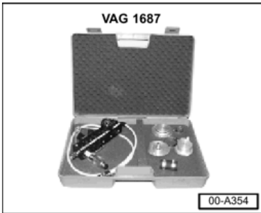
Fig. 218: Checking Charge Air Pressure System Using V.A.G 1687 Charge Air System Tester Courtesy of VOLKSWAGEN UNITED STATES, INC.
