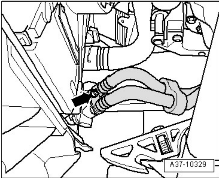
Fig. 63: Identifying Lines From Transmission Oil Cooler And Rear Mounting Bolts Courtesy of AUDI OF AMERICA, LLC
