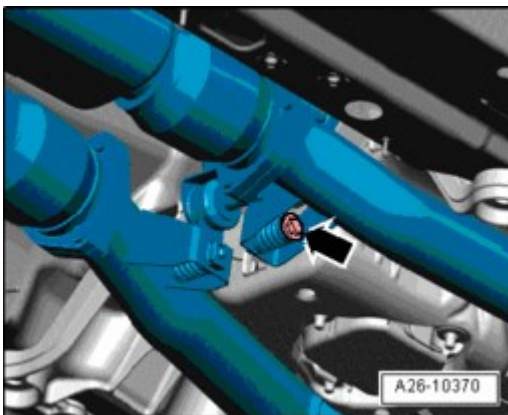
Fig. 91: Removing Bolt At Right Exhaust Tract Strap
