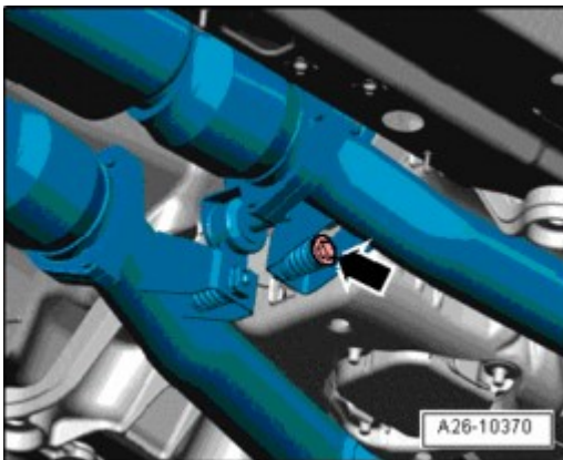
Fig. 558: Removing Bolt At Right Exhaust Tract Strap Courtesy of VOLKSWAGEN UNITED STATES, INC.
