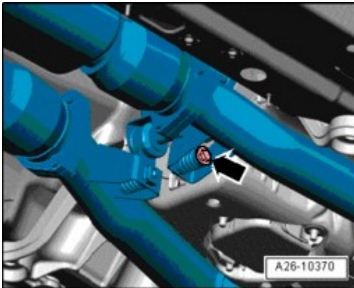
Fig. 102: Removing Bolt At Right Exhaust Tract Strap
