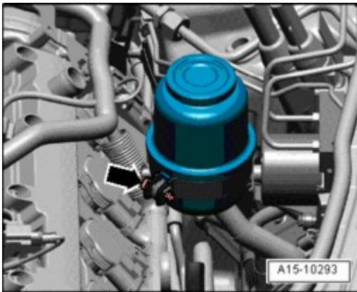
Fig. 288: Removing Bolt And Remove Power Steering Reservoir From Bracket, Hydraulic Lines Remain Connected Courtesy of VOLKSWAGEN UNITED STATES, INC.
