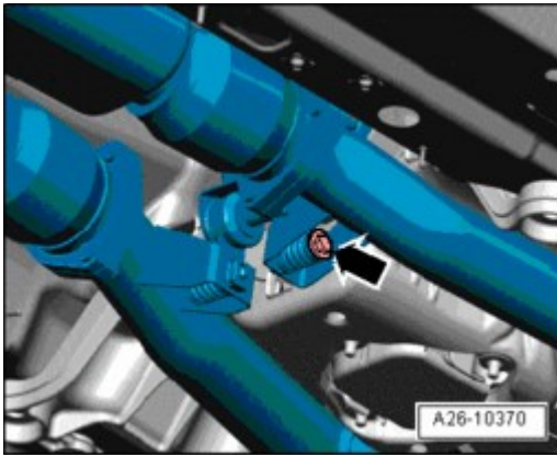
Fig. 529: Removing Bolt At Right Exhaust Tract Strap Courtesy of VOLKSWAGEN UNITED STATES, INC.
