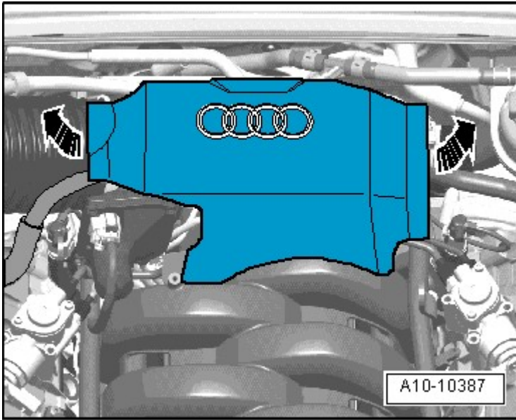
Fig. 544: Pulling Rear Engine Cover Off Courtesy of VOLKSWAGEN UNITED STATES, INC.
