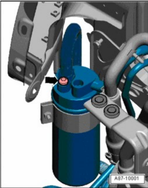
Fig. 74: Removing Bolt And Disconnecting Refrigerant Line To A/C Compressor Courtesy of VOLKSWAGEN UNITED STATES, INC.
