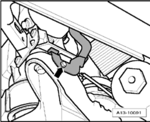
Fig. 407: Right Front Coolant Pipe Lower Bolt Courtesy of VOLKSWAGEN UNITED STATES, INC.
