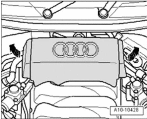
Fig. 574: Removing Rear Engine Cover
