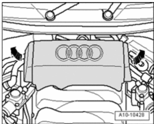
Fig. 587: Removing Rear Engine Cover
