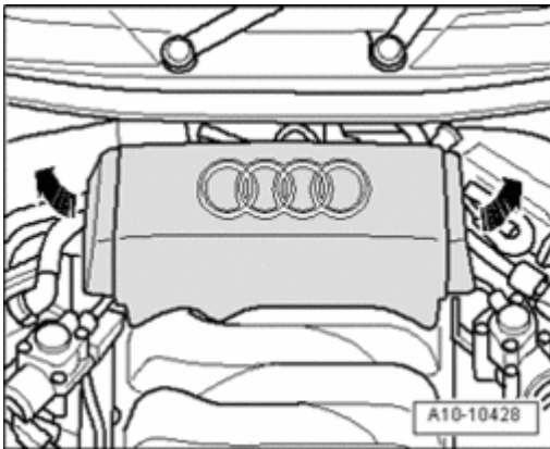
Fig. 17: Removing Rear Engine Cover Courtesy of VOLKSWAGEN UNITED STATES, INC.
