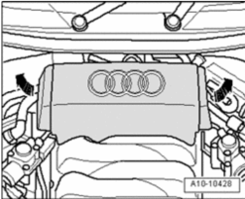
Fig. 574: Removing Rear Engine Cover
