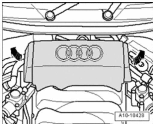
Fig. 126: Removing Rear Engine Cover Courtesy of VOLKSWAGEN UNITED STATES, INC.
