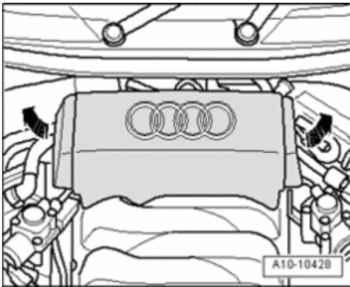
Fig. 562: Removing Rear Engine Cover
