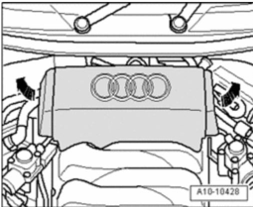
Fig. 590: Removing Rear Engine Cover
