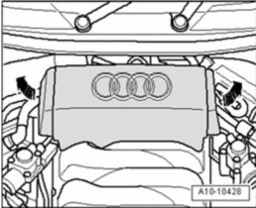
Fig. 592: Removing Rear Engine Cover
