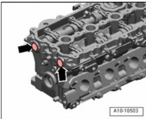
Fig. 365: Driving Sealing Plugs In Flush Courtesy of VOLKSWAGEN UNITED STATES, INC.
