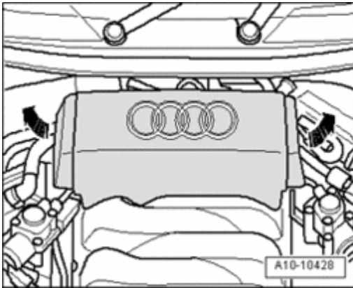
Fig. 471: Removing Rear Engine Cover
