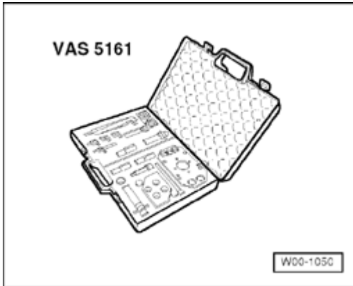
Fig. 441: Valve Cotter Disassembly/Assembly Device VAS 5161 Courtesy of VOLKSWAGEN UNITED STATES, INC.
