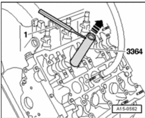
Fig. 326: Positioning Lower Part Of 3364 Valve Stem Removal Tool At Valve Stem Oil Seal Courtesy of VOLKSWAGEN UNITED STATES, INC.
