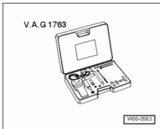
Fig. 170: Compression Tester VAG1381 Or VAG1763 Courtesy of VOLKSWAGEN UNITED STATES, INC.
