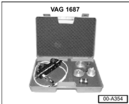
Fig. 295: Checking Charge Air Pressure System Using Vag1687 Charge Air System Tester Courtesy of VOLKSWAGEN UNITED STATES, INC.
