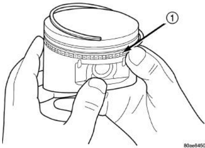
Fig. 247: Installing Piston Ring Side Rail Courtesy of CHRYSLER GROUP, LLC
