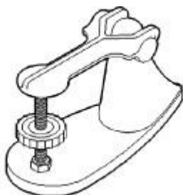
Fig. 127: Valve Spring Tester C-647 Courtesy of CHRYSLER LLC
