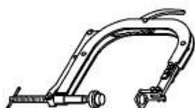
Fig. 34: COMPRESSOR, VALVE SPRING - C-3422-D
