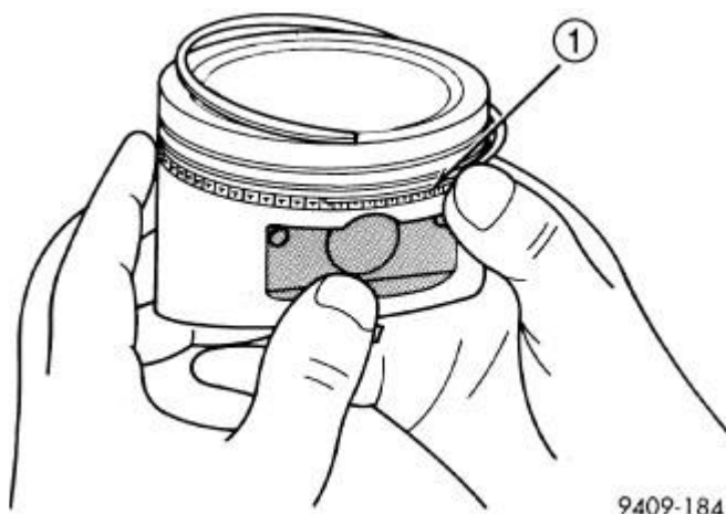
Fig. 211: Installing Side Rail Courtesy of CHRYSLER LLC
