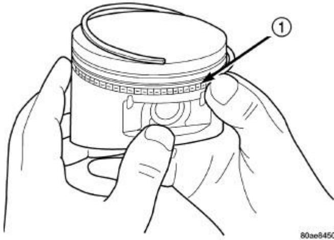
Fig. 445: Removing/Installing Piston Ring Side Rail Courtesy of CHRYSLER GROUP, LLC
