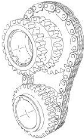
Fig. 647: Primary Chain, Idler Sprocket & Crankshaft Sprocket Courtesy of CHRYSLER GROUP, LLC
