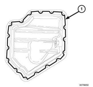
Fig. 537: Locating Sealant On Lower Oil Pan Courtesy of CHRYSLER LLC
