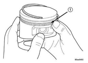
Fig. 432: Removing/Installing Piston Ring Side Rail Courtesy of CHRYSLER LLC
