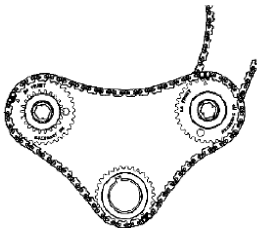
Fig. 860: Identifying Primary Camshaft Drive Chain & Large Sprockets Courtesy of SUZUKI OF AMERICA CORP.
