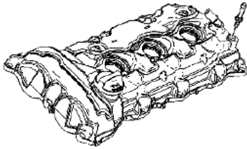
Fig. 536: Identifying Fuel Injector Sight Shield Ball Stud Courtesy of SUZUKI OF AMERICA CORP.
