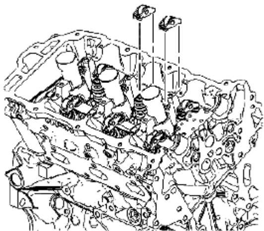
Fig. 370: Identifying Valve Rocker Arms Courtesy of SUZUKI OF AMERICA CORP.
