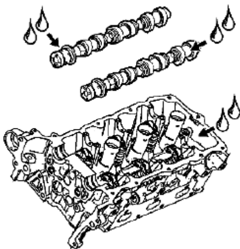
Fig. 767: Applying Liberal Amount Of Lubricant To Camshaft Journals & Left Cylinder Head Camshaft Carriers Courtesy of SUZUKI OF AMERICA CORP.
