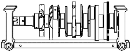
Fig. 408: Supporting Crankshaft With Suitable Fixture Courtesy of SUZUKI OF AMERICA CORP.
