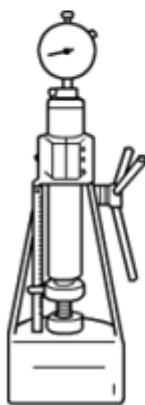
Fig. 132: Checking Valve Spring Free Length Courtesy of SUZUKI OF AMERICA CORP.
