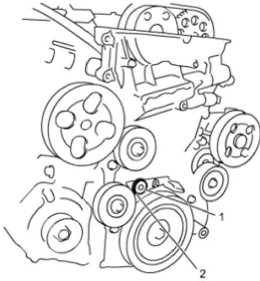
Fig. 32: Removing Timing Chain Cover Plug And Gasket Courtesy of SUZUKI OF AMERICA CORP.
