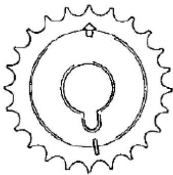
Fig. 71: Identifying Camshaft Sprocket Teeth Courtesy of SUZUKI OF AMERICA CORP.
