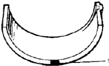
Fig. 156: Identifying Connecting Rod Bearing Courtesy of SUZUKI OF AMERICA CORP.
