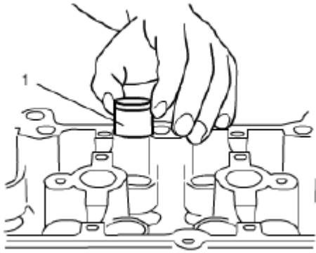
Fig. 93: Identifying Tappet & Shim Courtesy of SUZUKI OF AMERICA CORP.
