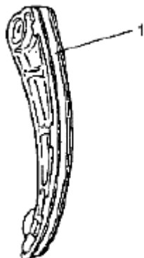
Fig. 86: Identifying Timing Chain Tensioner Shoe Courtesy of SUZUKI OF AMERICA CORP.
