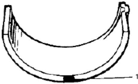
Fig. 192: Identifying Paint Mark For Standard Size Main Bearing Thickness Courtesy of SUZUKI OF AMERICA CORP.
