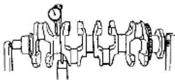
Fig. 183: Measuring Runout At Center Journal Courtesy of SUZUKI OF AMERICA CORP.
