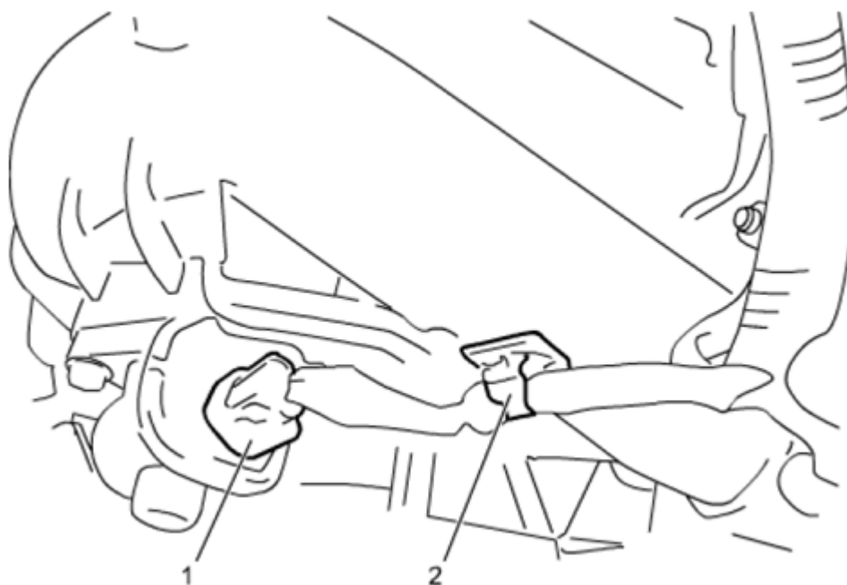
Fig. 28: Identifying IMT Valve Connector With Clamp Courtesy of SUZUKI OF AMERICA CORP.
