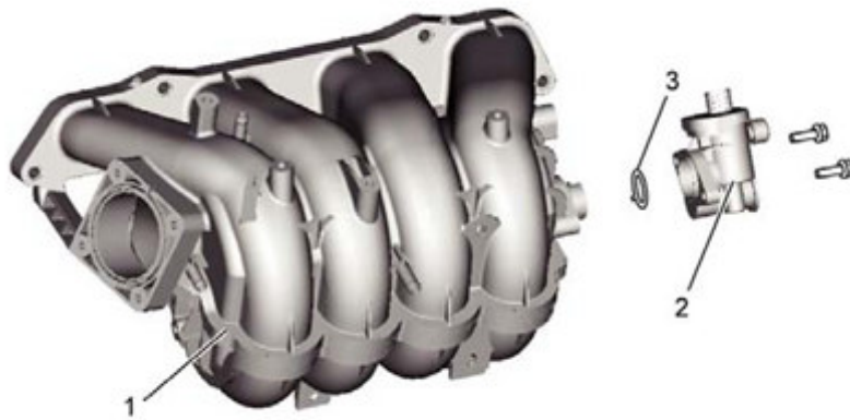
Fig. 23: Identifying IMT Valve Actuator And Gasket Courtesy of SUZUKI OF AMERICA CORP.
