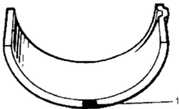
Fig. 174: Identifying Connecting Rod Bearing Mark Location Courtesy of SUZUKI OF AMERICA CORP.
