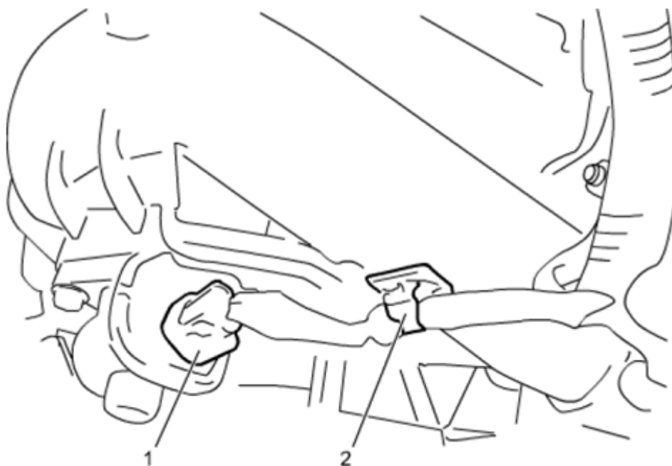
Fig. 33: Identifying IMT Valve Connector And Clamp Courtesy of SUZUKI OF AMERICA CORP.
