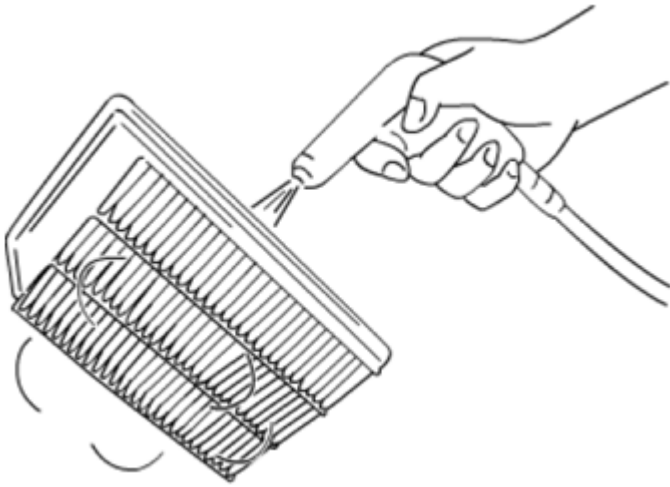
Fig. 11: Cleaning Air Cleaner Filter Courtesy of SUZUKI OF AMERICA CORP.
