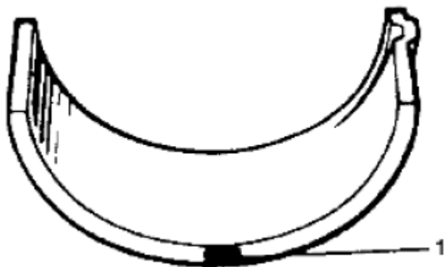
Fig. 172: Identifying Specified Colors For Identification On Connecting Rod Bearing Courtesy of SUZUKI OF AMERICA CORP.
