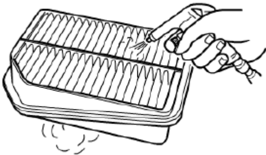
Fig. 20: Cleaning Air Filter
