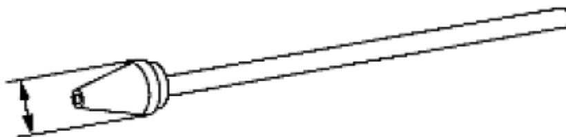
Fig. 20: Identifying Compression Gauge Diameter Courtesy of SUZUKI OF AMERICA CORP.
