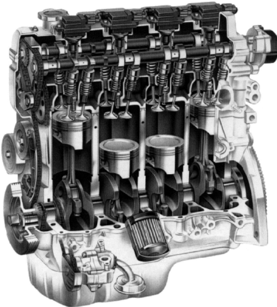
Fig. 1: Identifying Double Overhead Camshaft Valve Mechanism Courtesy of SUZUKI OF AMERICA CORP.
