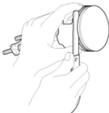
Fig. 31: Measuring Clearance Between Piston Ring And Wall Of Ring Groove Using Feeler Gauge Courtesy of HYUNDAI MOTOR CO.
