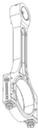
Fig. 14: Identifying Connecting Rod Mark Location Courtesy of HYUNDAI MOTOR CO.
