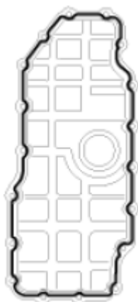
Fig. 49: Identifying Sealant Applying Area Of Lower Oil Pan Courtesy of HYUNDAI MOTOR CO.
