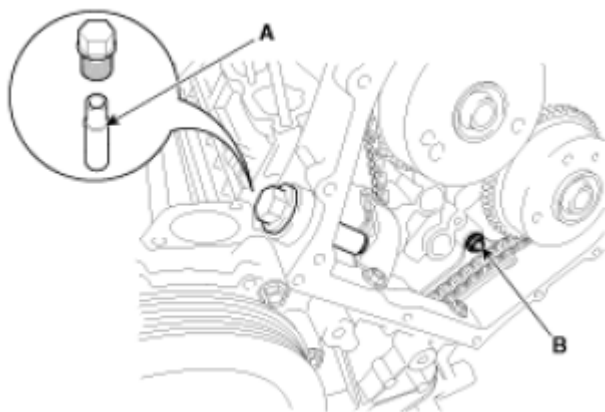
Fig. 59: Identifying Timing Chain Tensioner And Chain Guide Fixing Bolt Courtesy of HYUNDAI MOTOR CO.
