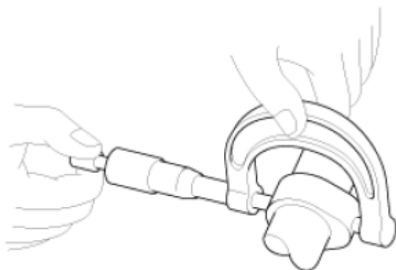
Fig. 82: Identifying Measure Cam Lobe Height Using Micrometer Courtesy of HYUNDAI MOTOR CO.
