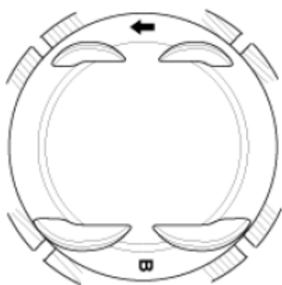
Fig. 35: Identifying Piston Installing Direction Courtesy of HYUNDAI MOTOR CO.
