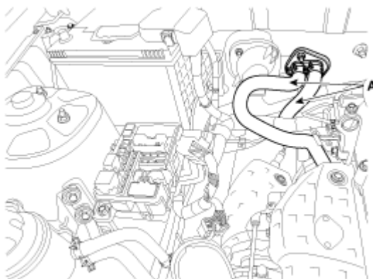
Fig. 45: Identifying Heater Hoses Courtesy of HYUNDAI MOTOR CO.
