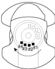
Fig. 11: Locating Crankshaft Pin Mark Courtesy of HYUNDAI MOTOR CO.
