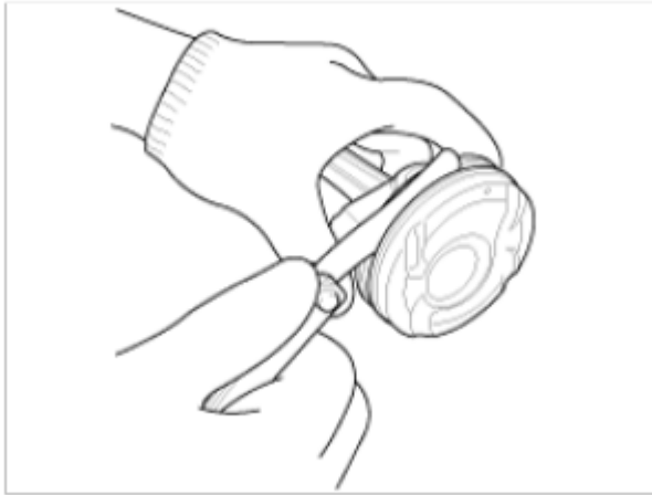
Fig. 25: Measuring Piston Ring Side Clearance Using Feeler Gauge Courtesy of HYUNDAI MOTOR AMERICA
