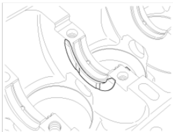
Fig. 32: Identifying Thrust Bearing Courtesy of HYUNDAI MOTOR AMERICA
