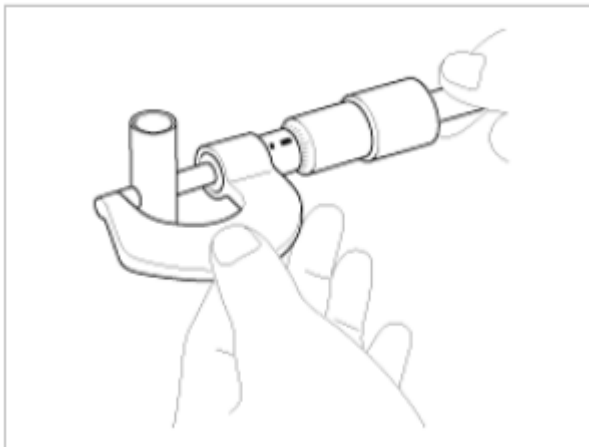
Fig. 27: Measuring Piston Pin Outer Diameter Using Micrometer Courtesy of HYUNDAI MOTOR AMERICA
