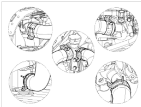
Fig. 83: Identifying Radiator Hose Installation Position Courtesy of HYUNDAI MOTOR AMERICA
