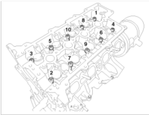
Fig. 34: Identifying Cylinder Head Bolts Loosening Sequence Courtesy of HYUNDAI MOTOR AMERICA
