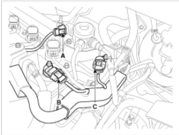
Fig. 8: Identifying Fuel Pressure Control Valve, Intake And Exhaust Camshaft Position Sensor Connectors
