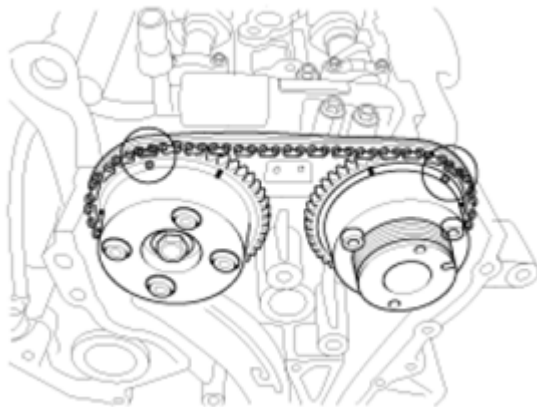
Fig. 10: Timing Chain And Sprocket Identification Mark (LH1) Courtesy of HYUNDAI MOTOR CO.
