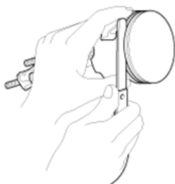
Fig. 30: Inspecting Piston Ring Side Clearance Using Feeler Gauge Courtesy of HYUNDAI MOTOR CO.
