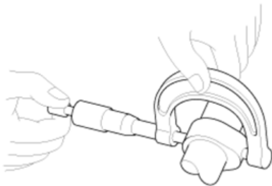
Fig. 22: Measuring Cam Lobe Height Using Micrometer Courtesy of HYUNDAI MOTOR CO.
