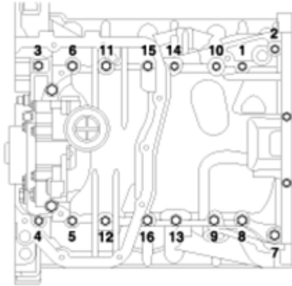
Fig. 50: Identifying Upper Oil Pan Bolts Courtesy of HYUNDAI MOTOR CO.
