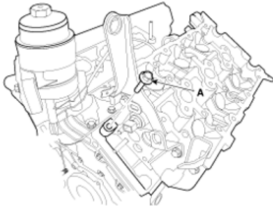
Fig. 10: Identifying RH Cylinder Head Rear Bolt Courtesy of HYUNDAI MOTOR CO.
