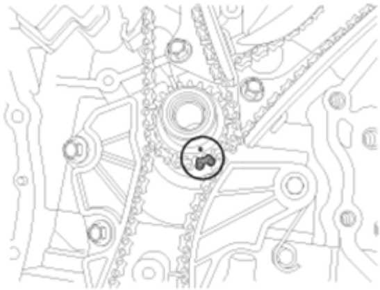
Fig. 9: Timing Chain And Sprocket Identification Mark (RH2) Courtesy of HYUNDAI MOTOR CO.
