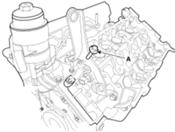
Fig. 44: Identifying Cylinder Head Bolt Courtesy of HYUNDAI MOTOR CO.
