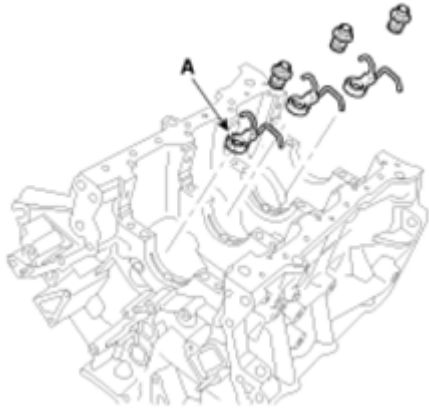
Fig. 11: Identifying Oil Jets Courtesy of HYUNDAI MOTOR CO.
