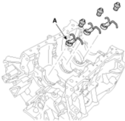
Fig. 36: Identifying Oil Jets Courtesy of HYUNDAI MOTOR CO.
