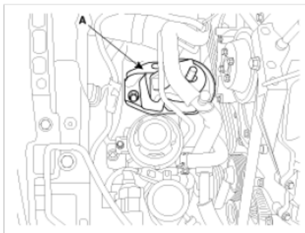
Fig. 142: Identifying No. 1 Engine Mounting
