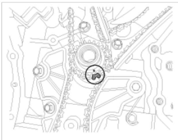
Fig. 105: Identifying Timing Mark On Intake Camshaft Sprocket And Exhaust Camshaft Sprocket
