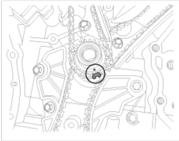
Fig. 74: Identifying Timing Mark On Sprocket And Timing Chain (2 Of 3)
