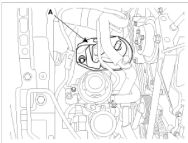
Fig. 46: Identifying No. 1 Engine Mounting
