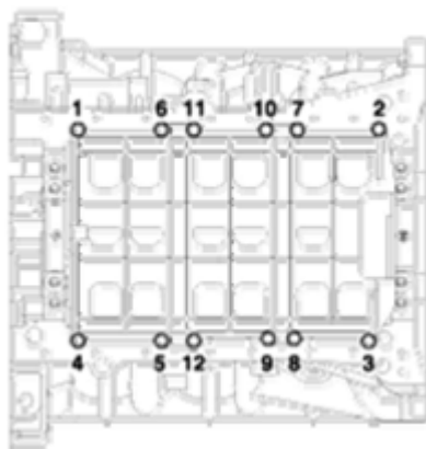
Fig. 46: Identifying Baffle Plate Bolts Tightening Sequence Courtesy of HYUNDAI MOTOR CO.
