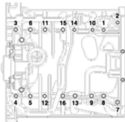
Fig. 48: Identifying Upper Oil Pan Bolts Tightening Sequence Courtesy of HYUNDAI MOTOR CO.
