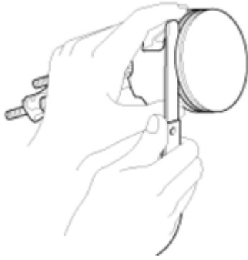
Fig. 28: Measuring Clearance Between Piston Ring And Wall Of Ring Groove Using Feeler Gauge Courtesy of HYUNDAI MOTOR CO.
