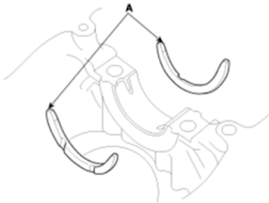
Fig. 35: Identifying Thrust Bearings Courtesy of HYUNDAI MOTOR CO.
