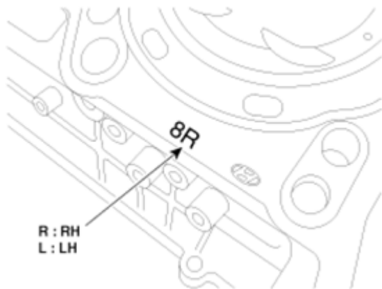
Fig. 28: Identifying Installation Direction Courtesy of HYUNDAI MOTOR CO.
