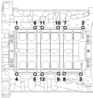
Fig. 46: Identifying Baffle Plate Bolts In Tightening Sequence Courtesy of HYUNDAI MOTOR CO.
