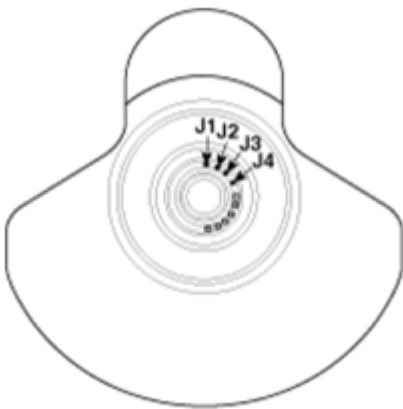
Fig. 19: Identifying Crankshaft Journal Mark Location Courtesy of HYUNDAI MOTOR CO.
