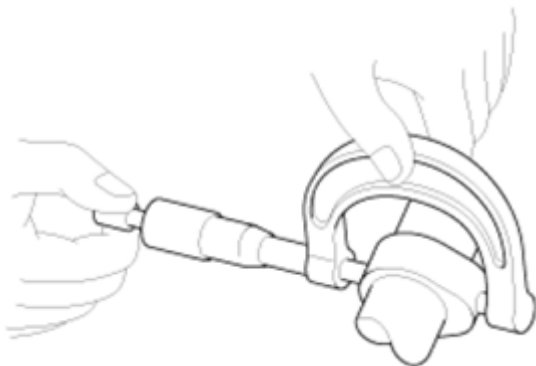
Fig. 15: Measuring Cam Lobe Height Courtesy of HYUNDAI MOTOR CO.
