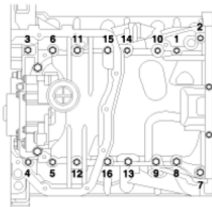
Fig. 48: Identifying Upper Oil Pan Bolts In Tightening Sequence Courtesy of HYUNDAI MOTOR CO.
