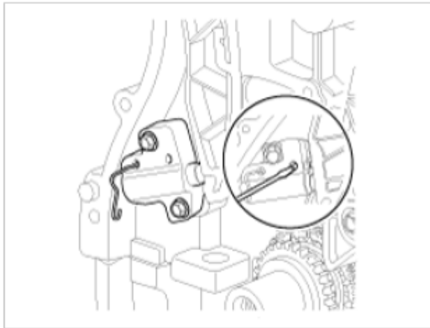
Fig. 93: Compressing RH Timing Chain Tensioner
