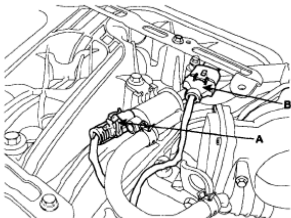
Fig. 321: Identifying PCSV Connector, MAP Sensor Connector And PCSV Hose Courtesy of HYUNDAI MOTOR CO.
