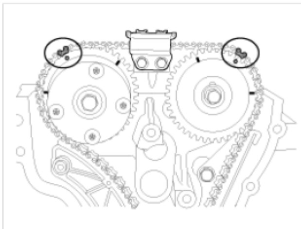
Fig. 113: Identifying Timing Chain Guide Sprockets Timing Mark
