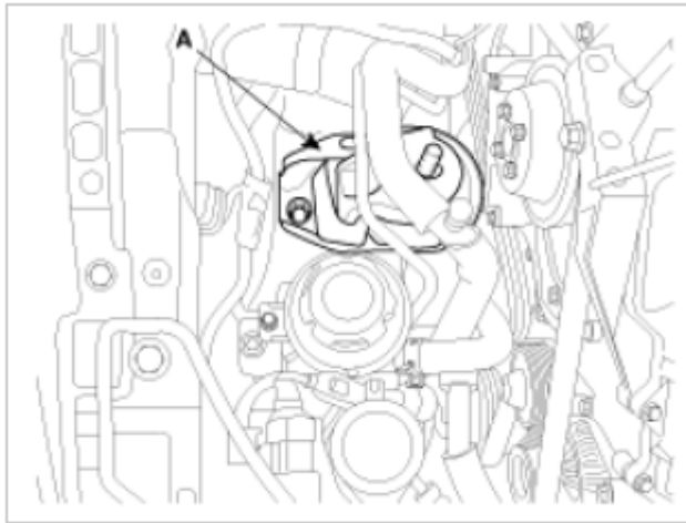
Fig. 53: Identifying No.1 Engine Mounting
