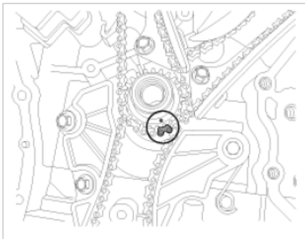
Fig. 121: Identifying Timing Chain Sprockets Timing Mark (2 Of 2)
