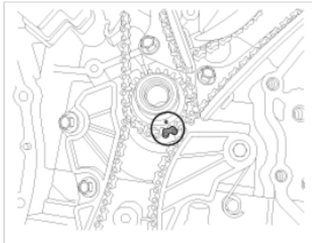
Fig. 90: Identifying Timing Chain Mark
