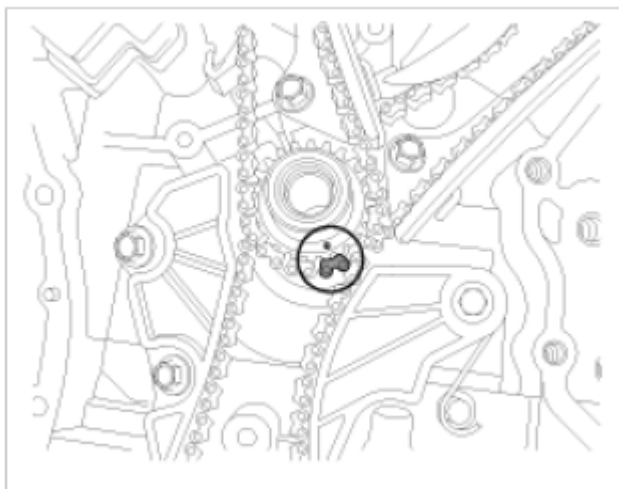
Fig. 25: Align Groove With Timing Mark "T" Of Timing Belt Cover Courtesy of HYUNDAI MOTOR CO.
