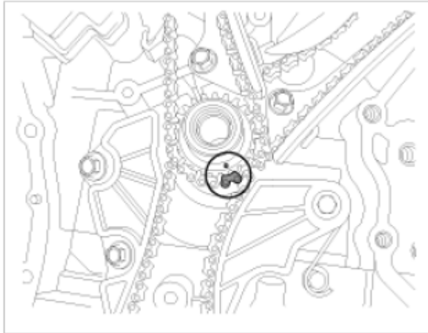
Fig. 240: Identifying Timing Marks Courtesy of HYUNDAI MOTOR CO.
