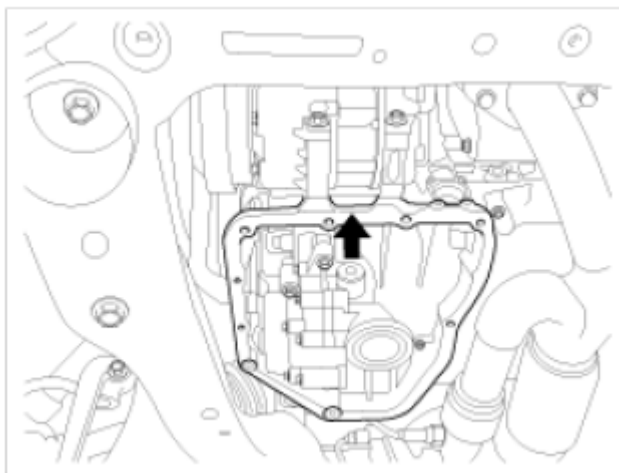
Fig. 227: Locating Timing Belt Upper Cover Courtesy of HYUNDAI MOTOR CO.
