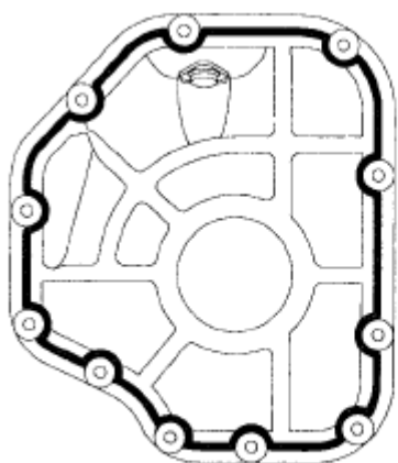
Fig. 116: Applying Liquid Sealant On Oil Pan Courtesy of HYUNDAI MOTOR CO.
