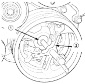
Fig. 37: Removing Damper Using Special Tools 8513 Insert And Tool 1026 Three Jaw Puller Courtesy of MITSUBISHI MOTOR SALES OF AMERICA.
