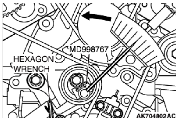
Fig. 107: Loosening Center Bolt Of Tensioner Pulley Courtesy of MITSUBISHI MOTOR SALES OF AMERICA.
