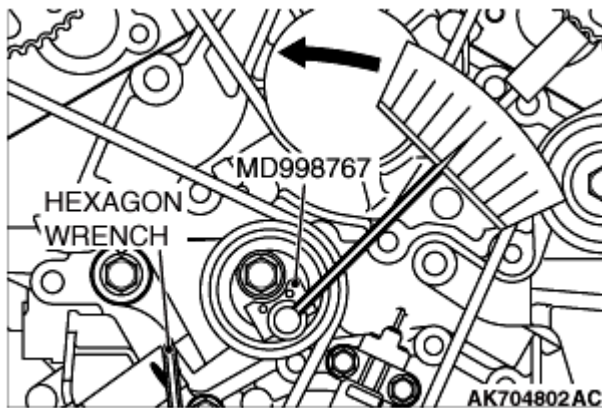
Fig. 96: Loosening Center Bolt Of Tensioner Pulley Courtesy of MITSUBISHI MOTOR SALES OF AMERICA.
