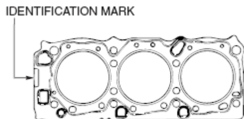
Fig. 99: Installing Cylinder Head Gasket
