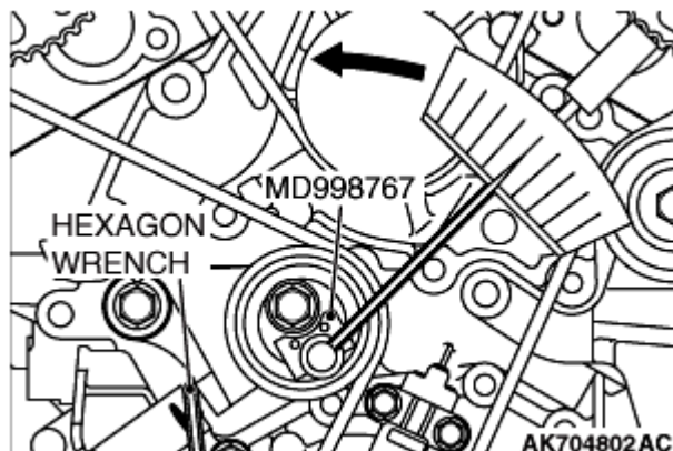
Fig. 118: Loosening Center Bolt Of Tensioner Pulley Courtesy of MITSUBISHI MOTOR SALES OF AMERICA.
