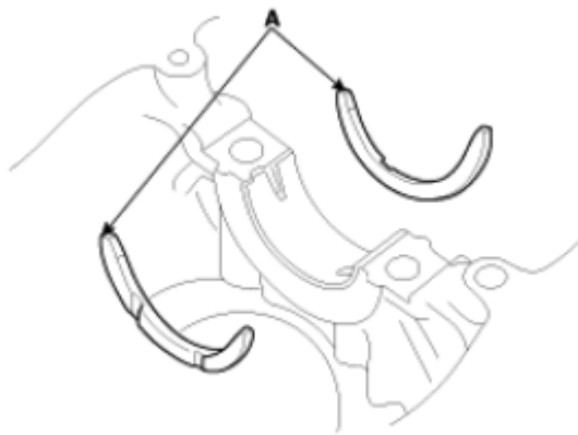
Fig. 85: Locating Thrust Bearings
