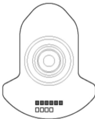
Fig. 47: Identifying Crankshaft Journal Mark Location Courtesy of KIA MOTORS AMERICA, INC.
