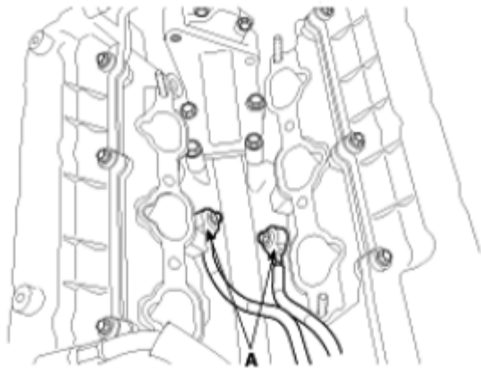
Fig. 12: Locating Knock Sensors
