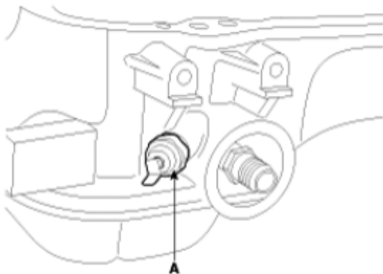
Fig. 77: Locating Oil Pressure Sensor Courtesy of KIA MOTORS AMERICA, INC.
