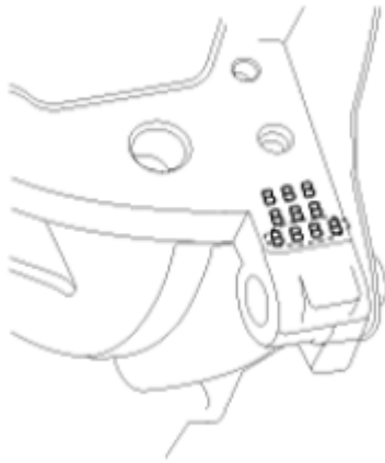
Fig. 25: Identifying Letters Stamped On End Of Block Courtesy of KIA MOTORS AMERICA, INC.
