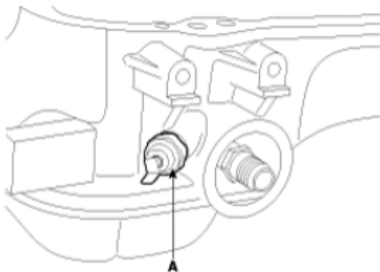
Fig. 96: Locating Oil Pressure Sensor Courtesy of KIA MOTORS AMERICA, INC.
