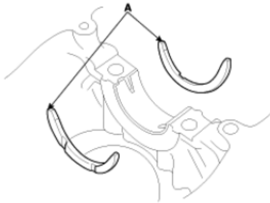
Fig. 66: Locating Thrust Bearings
