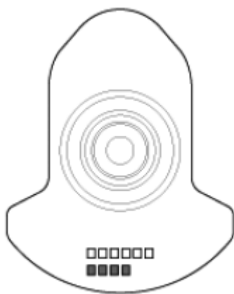
Fig. 22: Identifying Crankshaft Pin Mark Location Courtesy of KIA MOTORS AMERICA, INC.
